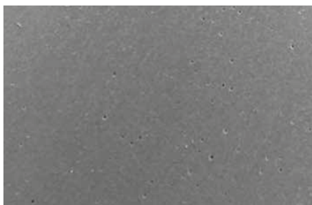
EFFECT OF 5 SEC AIR POLISHING ON GLASS IONOMER
